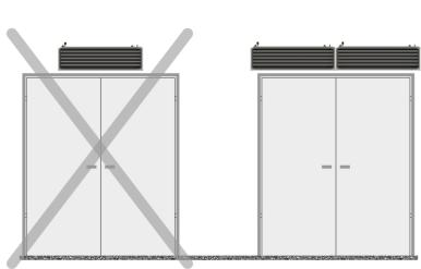
Width of doorway must be equal or lower than width of air curtain outlet (or outlets if air curtains are installed side by side).
