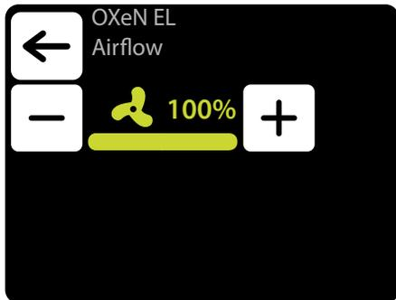
Appearance of this icon informs that the airflow setting has been defined in the weekly programmer. It is possible to change it ad hoc only. Change will only be active in given weekly programmer event.
