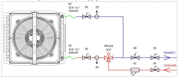
$\textbf{ZK-} \textbf{shut-} \textbf{off valve; } \textbf{ZO-} \textbf{vent valve; } \textbf{ZD-} \textbf{drain valve; } \textbf{FS-} \textbf{mesh filter; } \textbf{ZR-} \textbf{balancing valve; } \textbf{ZN-} \textbf{valve; } \textbf{valve; } \textbf{ZN-} \textbf{valv$
